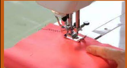
Machine stitching is a sewing stitch made by a sewing machine, sometimes using more than one thread.
