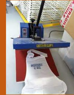
A heat press is a machine engineered to imprint a design or graphic on a substrate, such as a t-shirt, with the application of heat and pressure
