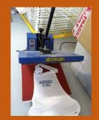
A heat press is a machine engineered to imprint a design or graphic on a substrate, such as a t-shirt, with the application of heat and pressure
