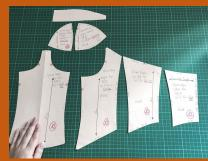
Pattern cutting in the fashion industry is the process of taking a design and making it into fabric. But before it is made into fabric, it is made into paper (2D).
